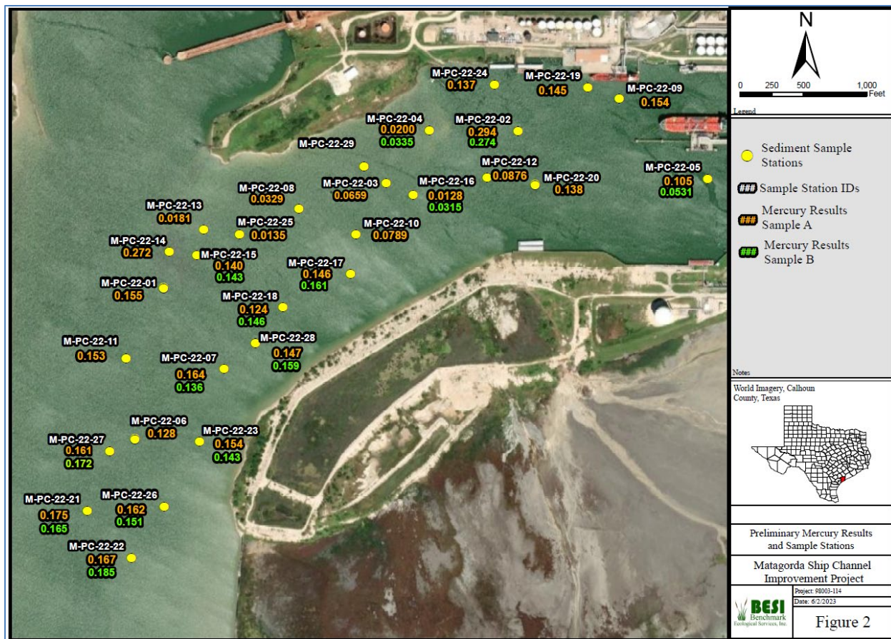
Figure 43 - 2023 Sediment sampling results for mercury (from 2023 report by BESi, Figure 2)
